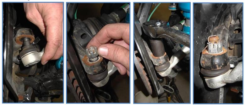
17. <u>Reconnecting brake and ABS line brackets</u>: Refer to step 9 for trimming brackets if you haven't already done so. Reinstall the trimmed brake line bracket to the steering knuckle upright using the factory bolt and tighten to 9 ft-lbs. Reconnect the bracket at the frame and tighten to 9 ft-lbs.
