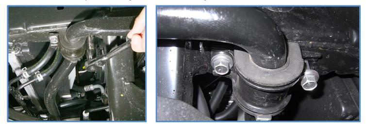
21. <u>Prepare the reservoir brackets for installation:</u> Install the reservoir clamps onto the reservoir bracket using the 1/4 X 1/2" BHCS (CB2420) provided in the kit. Use red locktite and tighten with a 5/32 Allen wrench. Keep in mind the reservoir brackets are side specific, do one side first then repeat steps 20-23 on opposite side.
