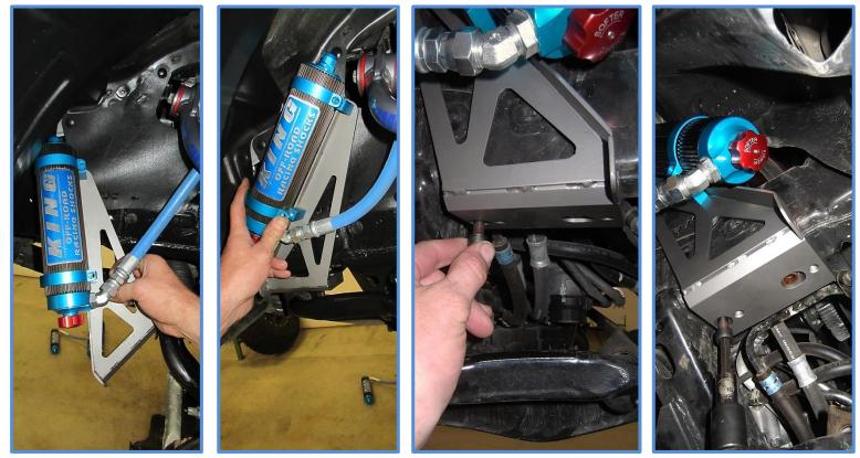
23. Bolt the sway bar to the bottom of the reservoir bracket using the supplied 3/8 X 3/4" bolts (CB4702). Tighten bolts to 35 ft-lbs. Repeat steps 20-23 on opposite side of vehicle. Reinstall skid plate after both sides are done.
