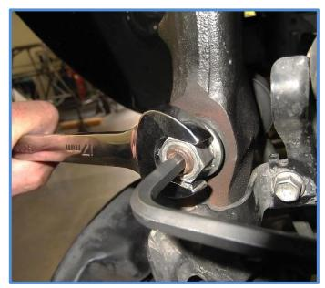
4. Pull the pin from the upper ball joint, loosen nut using a 19mm Socket and separate upper control arm from the steering knuckle.
