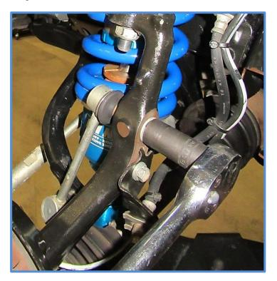
25. Center the reservoir in the clamps and install the 1/4 X 1" SHCS (CB1501). Tighten clamps with a 3/16 Allen wrench.
