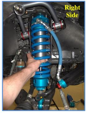
11. Install the factory lower mounting bolt in the lower mount as shown below. Place the washer and nut on the bolt but leave loose for now.
