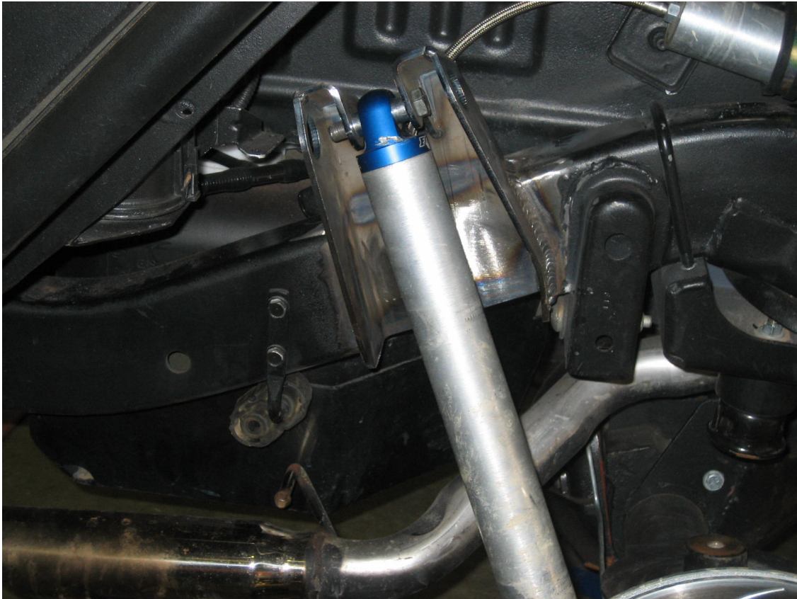
Side view of shock mount modification for track bar bracket.
